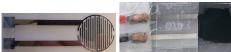
Figure 4.14: gas sensor (a) before adding PANi layer, (b) with PANi layer. The area outside the comb structure is covered with scotch tape (3M).
