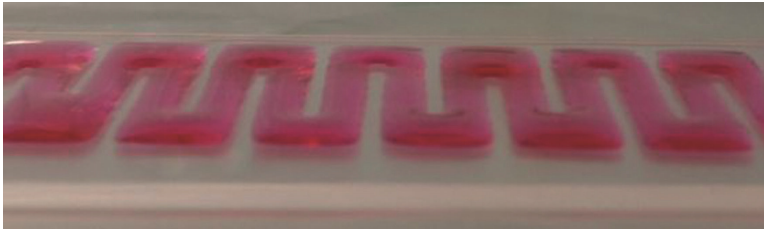
Figure 1.1: An example of the change in wettability created by patterned plasma treatment. A monolayer of dodecyl-trichlorosilane (DTS) has been deposited on glass to create a hydrophobic surface. Locally this DTS-layer was removed by patterned atmospheric plasma treatment to create a hydrophilic channel. Liquid placed on the substrate will wet the channel, but not the hydrophobic DTS-layer. The experimental work for this figure was carried out by Tom Vercoulen.
