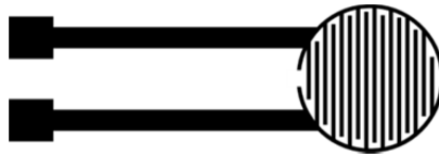
Figure 4.12: Schematic drawing of the electrodes of the chemresistor (Dimensions after printing 4.5x 2.0 \text{cm}^2 ).
