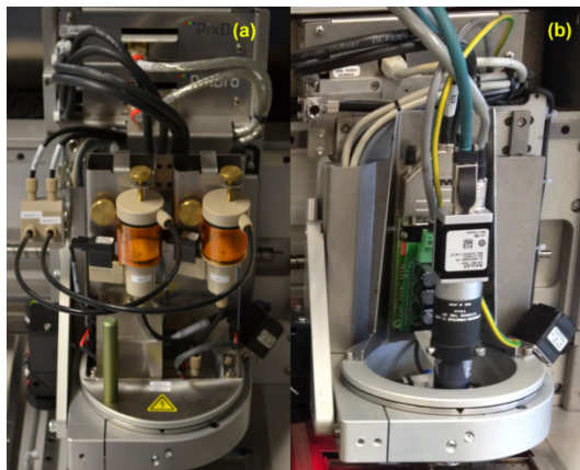
Figure 2.23: (a) Dimatix Spectra dualhead inkjet print head, (b) Innophysics POD24 plasma print head.
